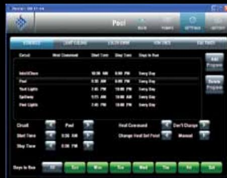
The Schedule screen shows circuit start and stop times to manage lights, heaters, spa jets and filter pumps.
