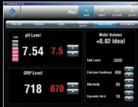
The IntelliChem® chemical controller interface enables customers to monitor their pH and sanitizing levels from their controller, rather than visiting the equipment pad. Compatible with Pentair's IntelliChlor salt chlorine generators, liquid feed pumps and CO<sub>2</sub> systems.
