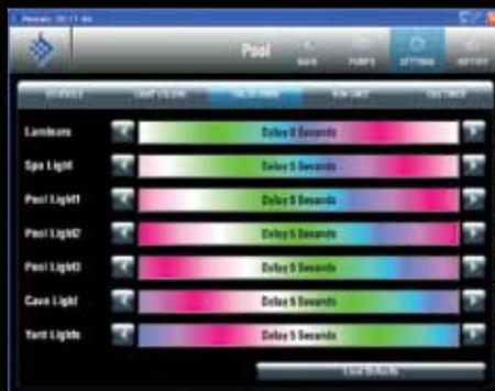
The Configure Swimming Colors screen displays control options for pool and spa lighting, as well as advanced configuration for IntelliBrite® 5g, SAm®, SAL® and FIBERworks® color lighting and landscape systems. It also allows control over advanced configurations for Color Set™, Color Swim™ and Color Sync™ lighting programs.
