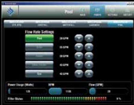
The IntelliFlo interface enables the IntelliTouch system to act as the master controller for up to four IntelliFlo Variable Speed pumps, eight IntelliFlo VF pumps, or combinations of both (maximum of four VS-3050 models).
